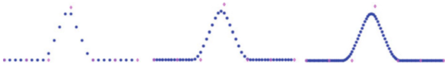
Fig. 16 Three steps of the scheme with masks (14) with n the subdivision level (initial points in magenta)
